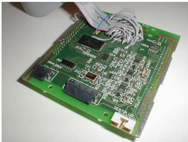
Bottom: An OTP PROM in the flight version replaces the ribbon cable.
