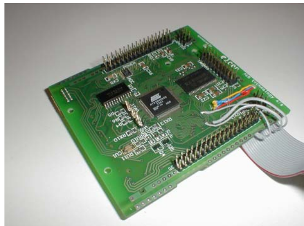
Top: The IDC connectors are mounted at the top for testing purpose only. In the flight version they must be at the bottom.
