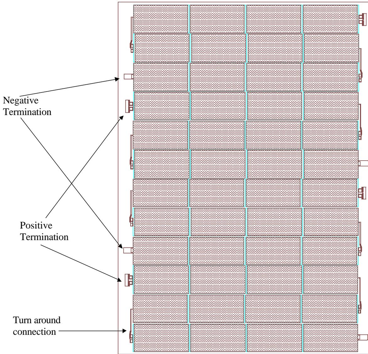
Figure 1-9 Solar Array Surface Layout of Side Panel
