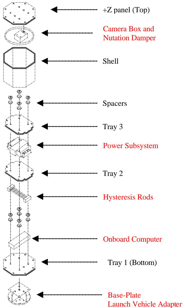
Figure 1-2 Satellite Exploded View with Launch Vehicle Adapter
