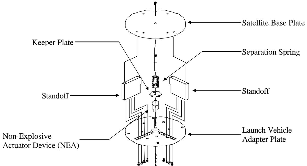
Figure 1-3 Exploded View of Launch Vehicle Adapter
