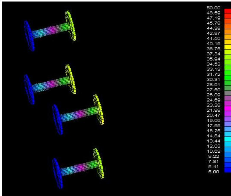
Fig. 1-11 Simulated Heat Load on Spartnik’s Spacers
