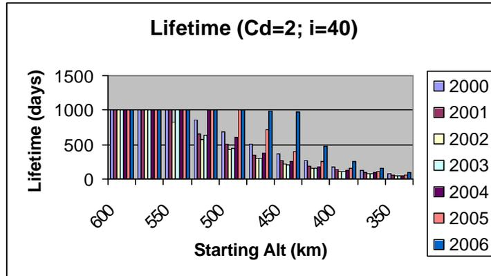
Figure 1-1: Orbital Lifetime vs. Starting altitude and year of Epoch
