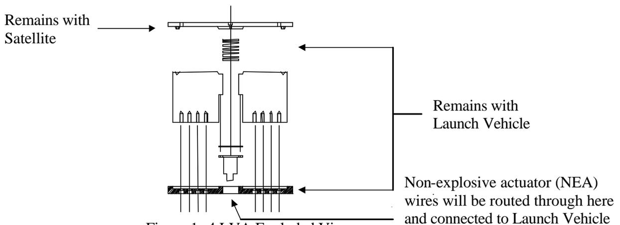
Figure 1- 4 LVA Exploded View
