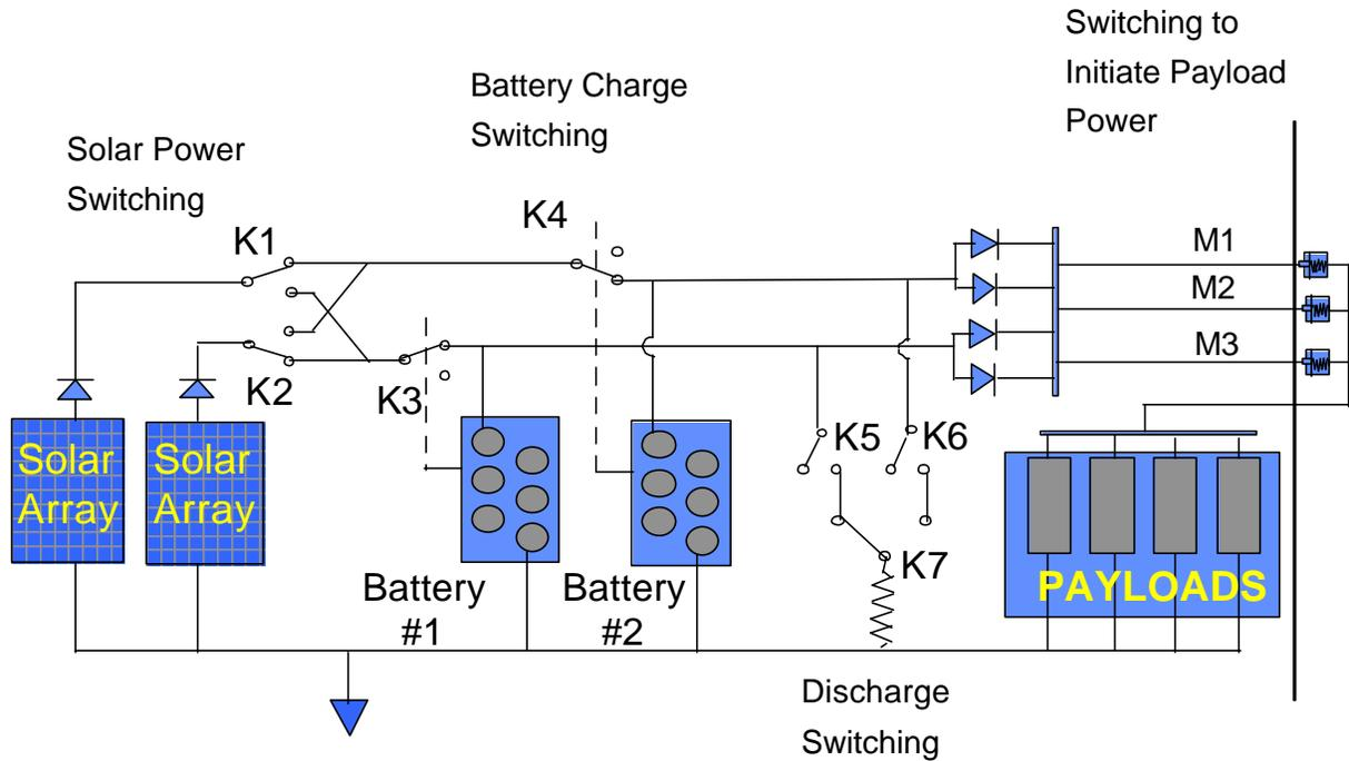
Figure 1-8 Power Wiring Configuration
