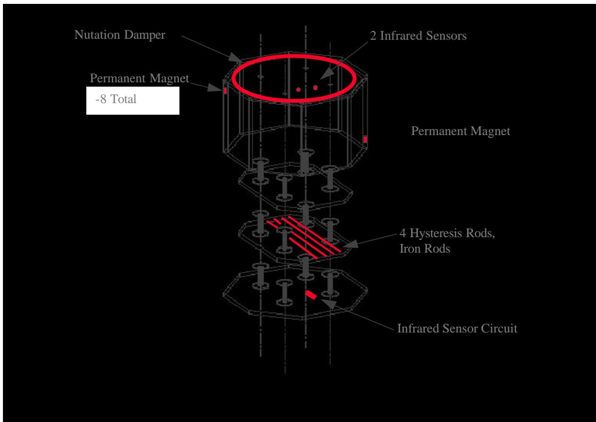
Figure 1-6 Attitude Determination and Control Hardware Locations
