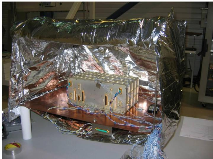
Figure 3.19: Insulating MLI blanket covering up the whole set-up
