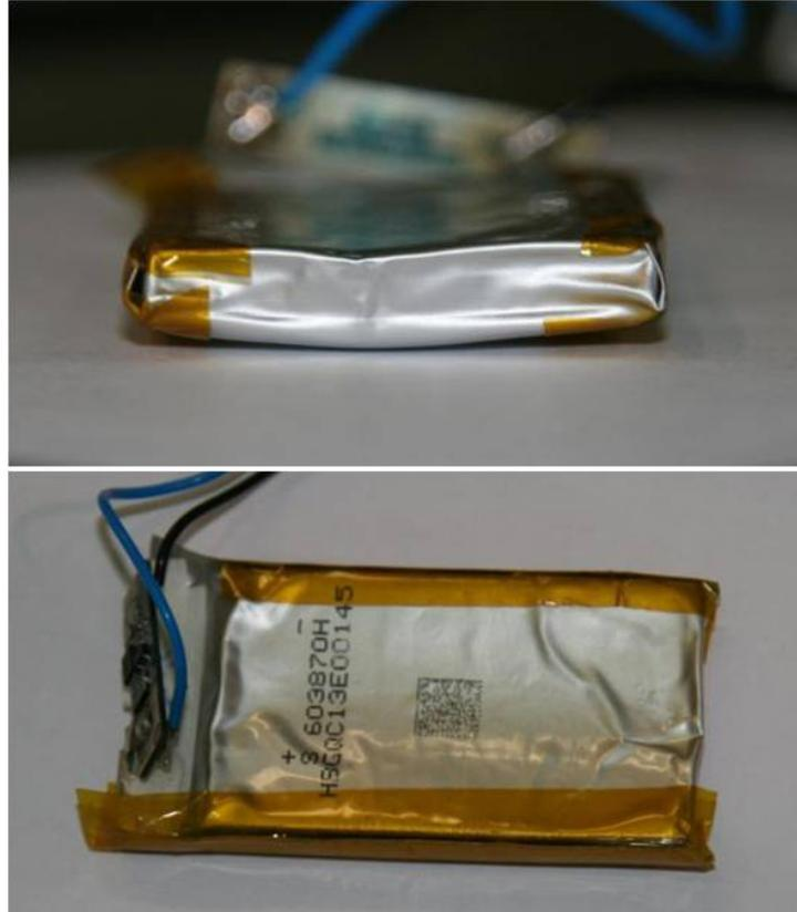
Figure 2.3: Deformation state exhibited under vacuum by KOKAM battery (*KOKAM SLB 603870H*) : the battery twists (top Figure) and crinkles (bottom Figure)
