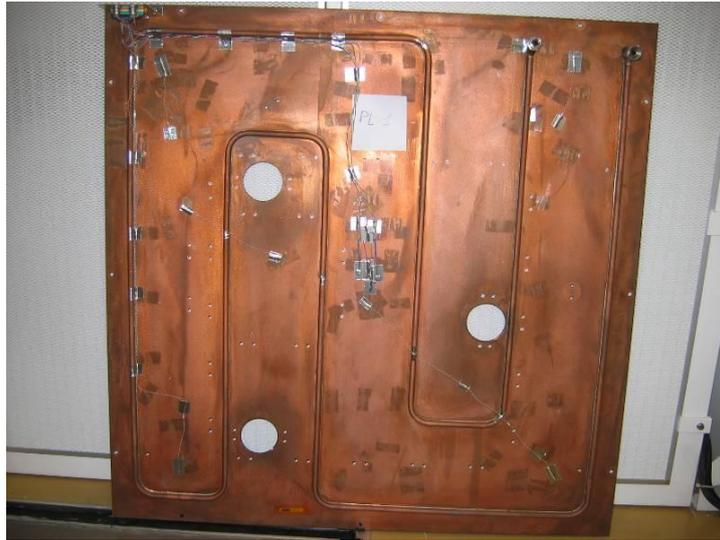
Figure 3.15: The copper temperature-controlled panel (rear side) and the brazed heating coil
