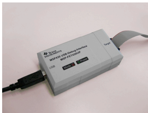
Figure 11.1: Texas Instruments' JTAG interface used to program and debug OBC1 and OBC2.
