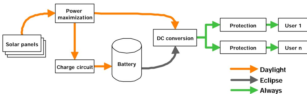
figure 3 - Architecture of the power system
