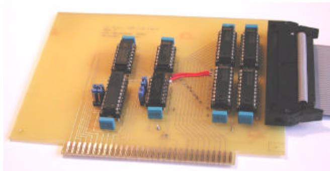
*Figure D.1 - The ISA data acquisition card*
