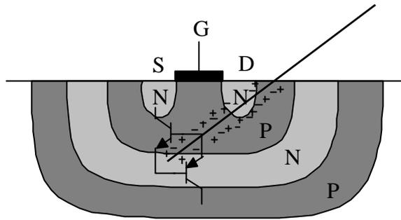
figure 18 - High energy particle hitting an N-MOS transistor (rough outline)
