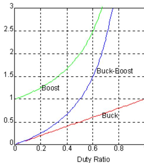
figure 28 - Duty cycles vs. voltage ratios for switching DC/DC converters
