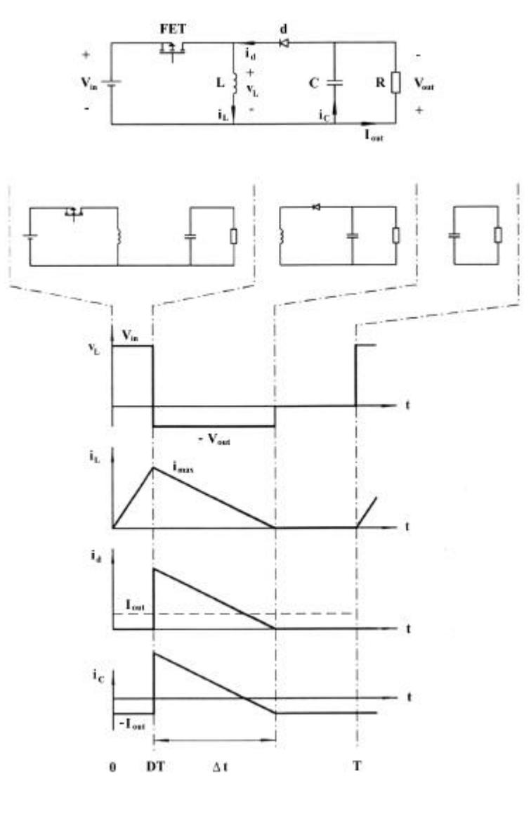
figure 25 - Buck boost in discontinuous conduction mode
