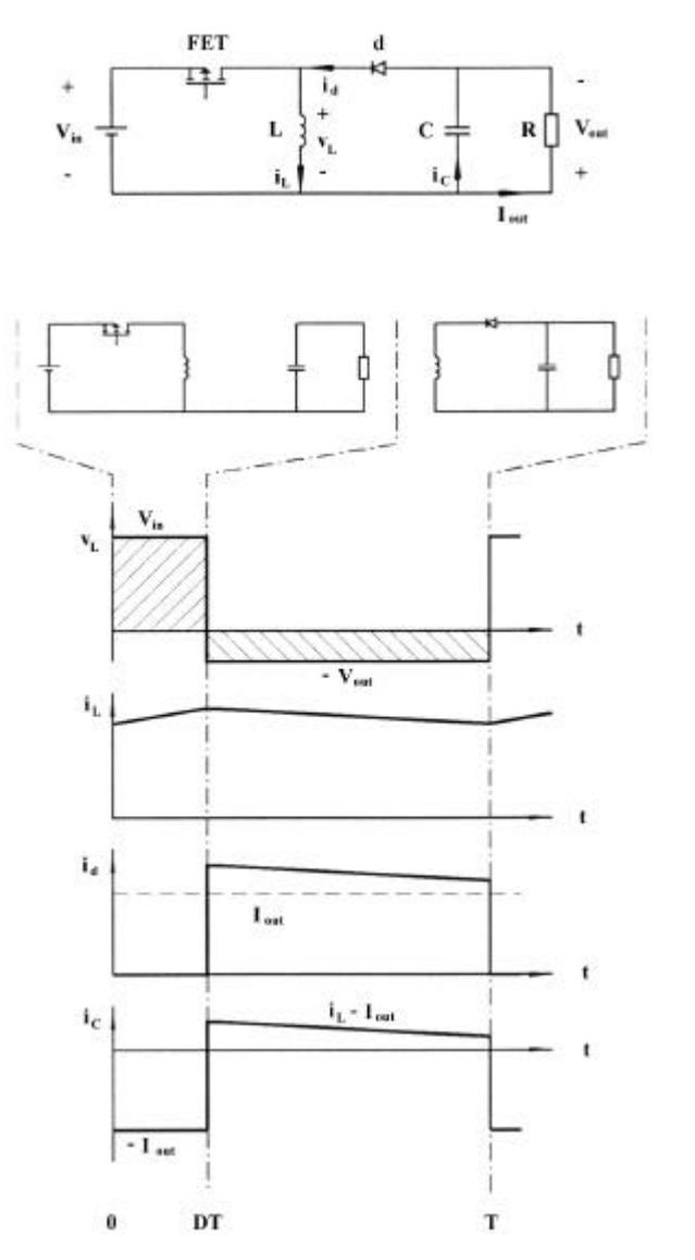
figure 24 - Buck-boost converter in continuous conduction mode
