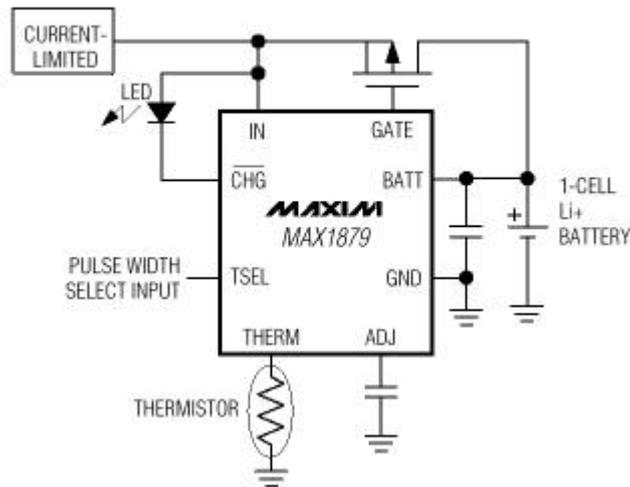
*figure 23 - Typical operation circuit for the Max1879 Li charger*
