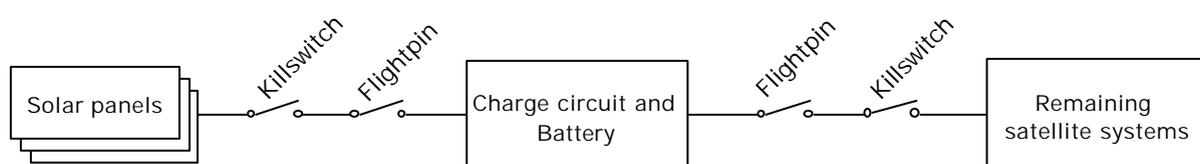
figure 2 - Overview of kill switches and flight pins
