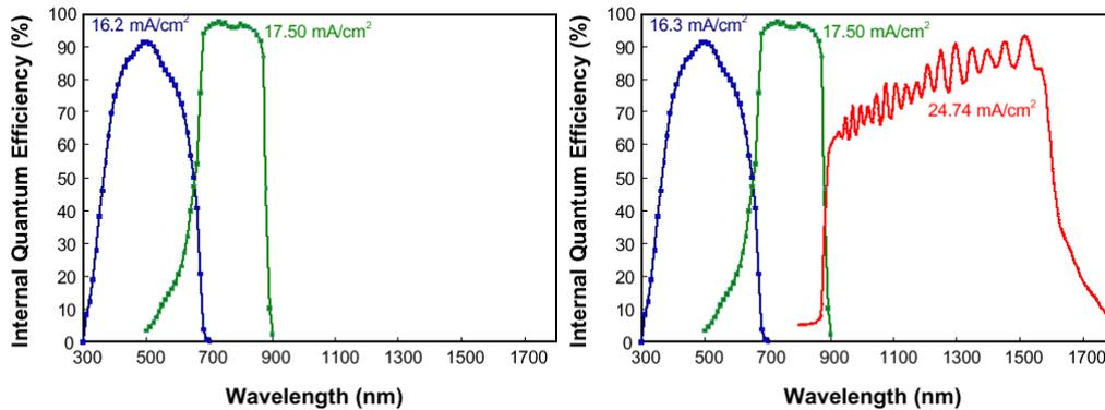
figure 5 - Internal Quantum Efficiency for Emcore's dual junction cells (left), and triple junction cells (right)
