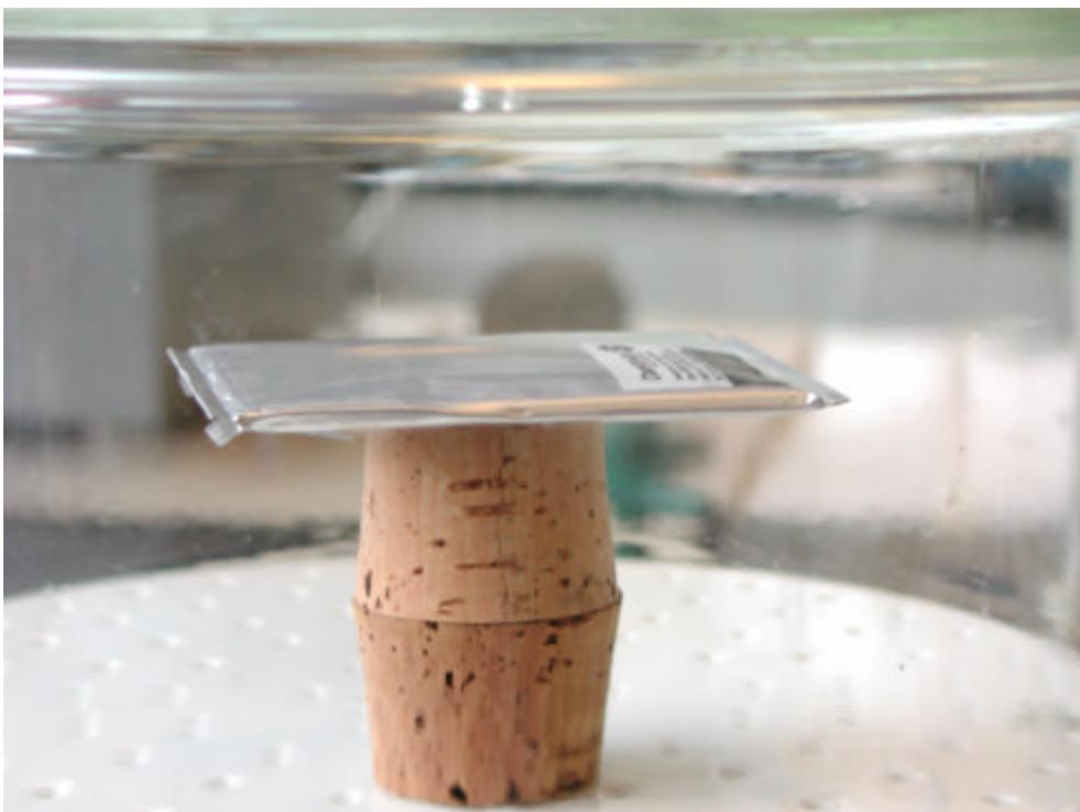
*Figure G.2 - The battery swelled up during the test at  $10^{-5}$  Torr*
