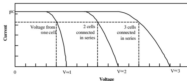
figure 8 - Serial connection of cells with the same level of illumination
