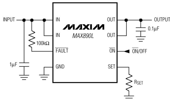
figure 31 - Typical operating circuit of the Max890
