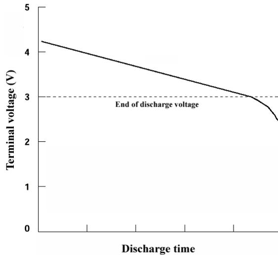
figure 17 - Discharging profile of a Li-Ion or a Li-Ion Polymer battery
