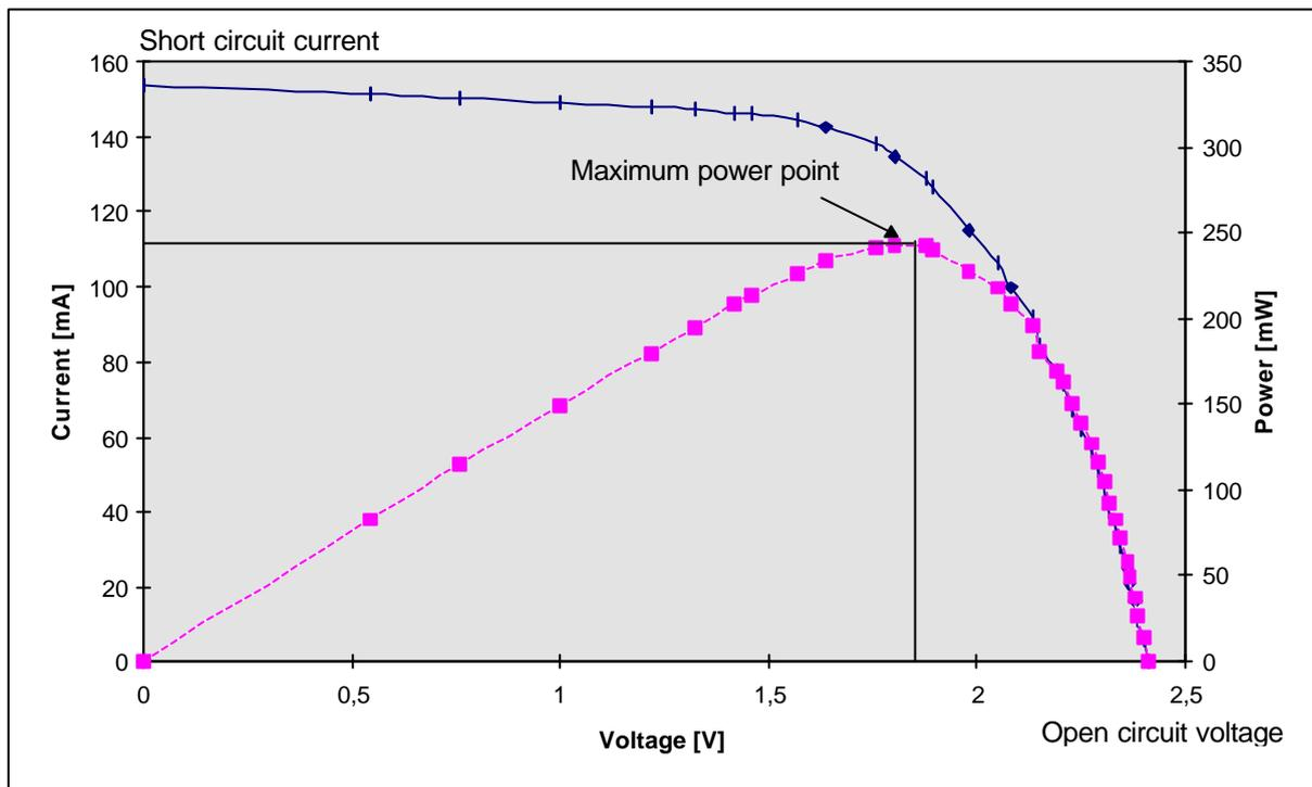
It is evident that  $I_{SC}$  is less than the specified 200 mA, a more correct value would be 150 mA, also we can estimate  $U_{OC} = \frac{2,4V}{5} = 0,48V$ , which is pretty much the specified value.
