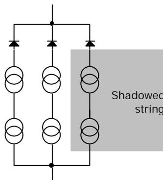
figure 9 - Use of blocking diodes
