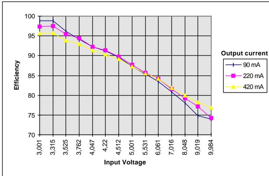
figure 30 - Efficiency test of Max1626
