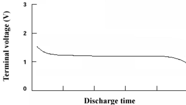
*figure 13 - Discharge profile for a NiCd or NiMh cell*
