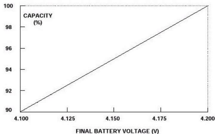
figure 16 - Effect of undercharge on Li-Ion and Li-Ion polymer battery capacity where the final voltage is 4.2V
