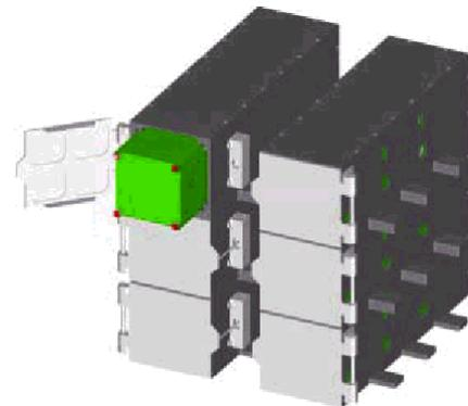
figure 1 - 6 P-PODs each containing 3 Cubesats
