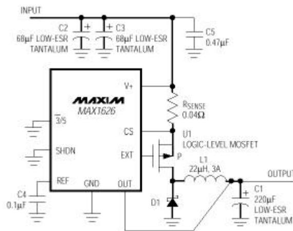
figure 29 - Typical application circuit for Max1626
