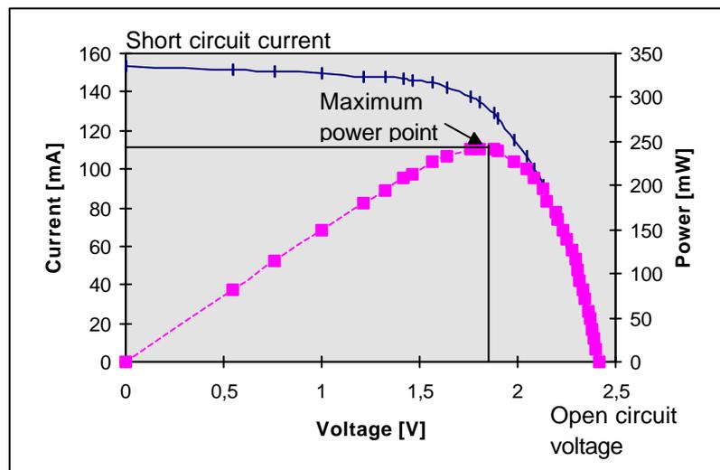
figure 6 - I/V characteristics of a solar cell
