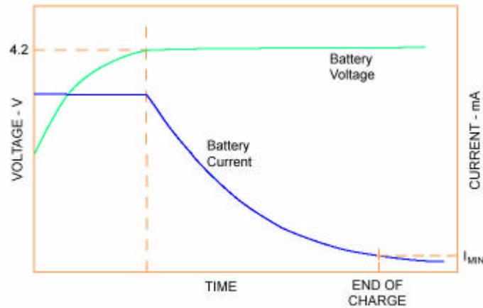
figure 15 - Li-Ion Battery charging characteristic for a battery with a final voltage of 4.2V
