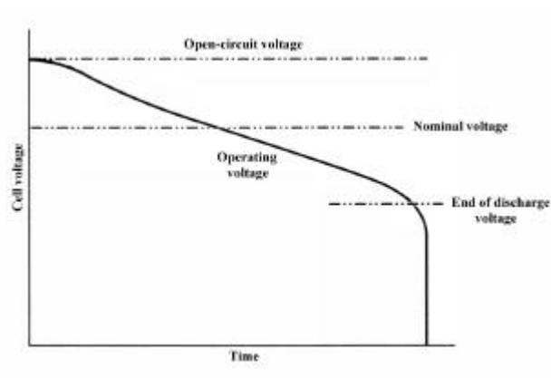
figure 11 - Voltage characteristics of a battery
