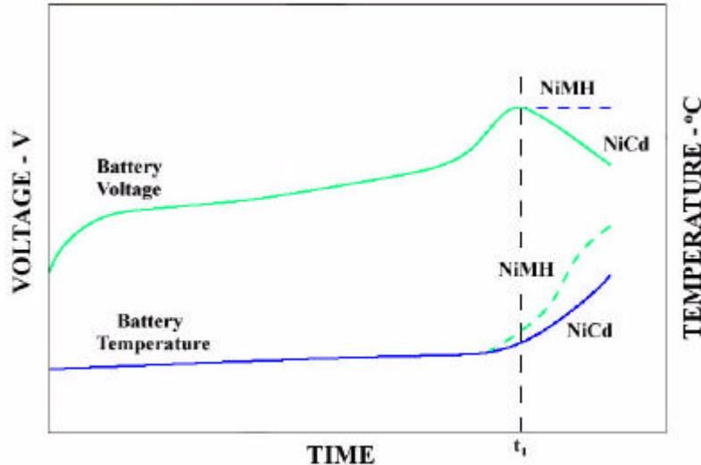
figure 12 - NiCd and NiMH charging characteristic
