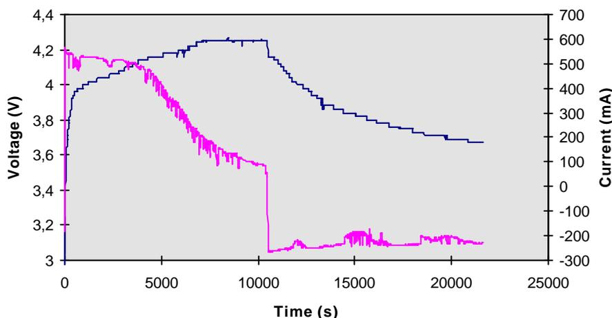
figure 22 - Charge and discharge cycle for the Danionics Li-Ion polymer battery
