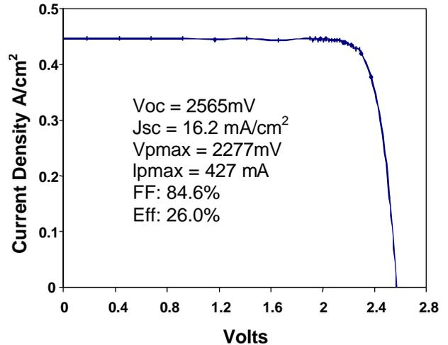
**Flight cell Beginning-of-Life efficiency for any shipment to range from 24.5% to 28%**
