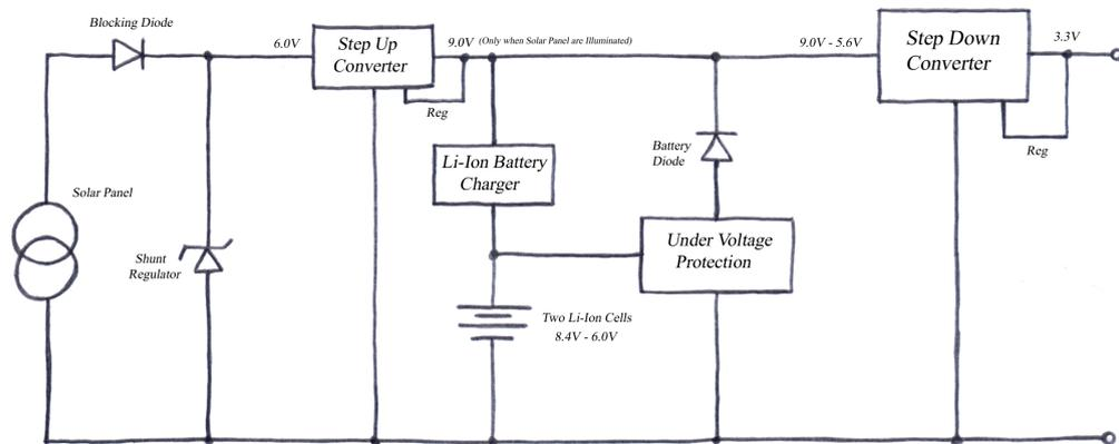
To charge two series connected Li-Ion batteries requires at least 9 V, and the Li-Ion charger has to control the individual battery cell voltages to prevent overcharging because even though the total voltage of the series connected batteries is lower than 8.4V the voltage of one of the cells can exceed 4.2V and therefore become overcharged. This makes the charging circuit more complex than the single cell charger, but if a single chip solution is chosen the designer won't see much difference.
