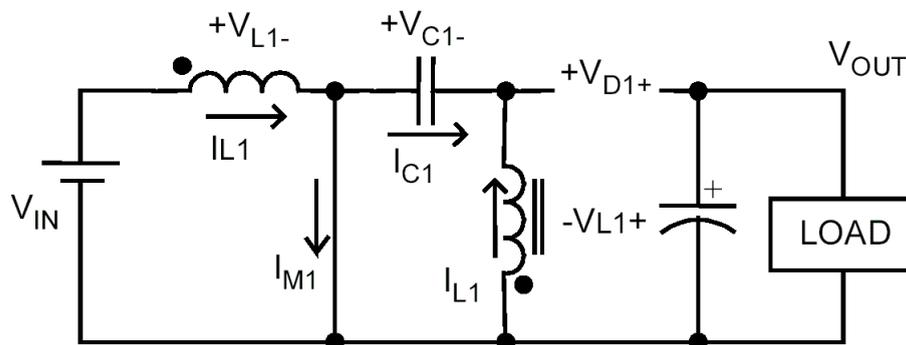
The input voltage  $V_{IN}$  is across the inductor  $L_1$  and the current in  $L_1$  increases in linear proportion.
