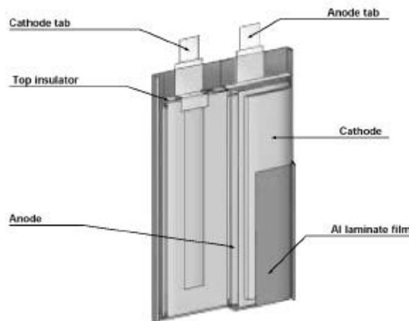
The cell is packed at low pressure but when the cell is brought into space where the pressure is even lower the cell will swell because of the few air molecules that are inside the foil packaging. If the molecules are inside the battery and not just between the outer Al laminate film and the battery, the swelling will cause the battery to lose capacity. Only tests can determine if the polymer battery can be used for space applications.
