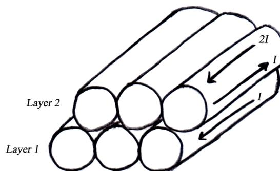
To find the ac resistance of the wire Jongsma's model can be used. It states that the ac resistance is the dc resistance times a corrections factor  $F_R$ . This factor can be found by the following equation.
