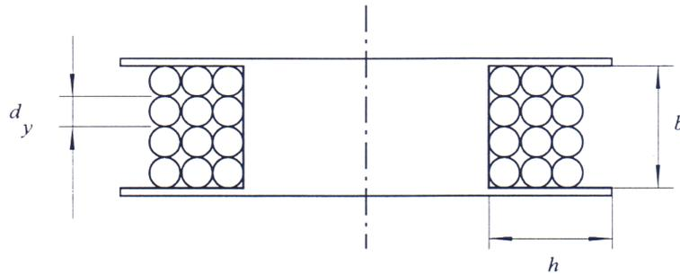
The largest outer diameter  $d_y$  of the copper wire is determined by the available winding space  $A_v = b \cdot h$ . To account for all the air between the windings, the wire is assumed to be quadratic with a side length equal to the outer diameter of the copper wire. Then the available winding space can be used to find the largest outer diameter of the wire:
