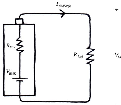
A battery can be seen as an electromotive force  $V_{EMK}$  in series with an equivalent series resistance  $R_{SER}$ . The electromotive force can be described as
