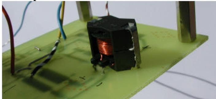
This is the battery charging / undervoltage protection circuit:
