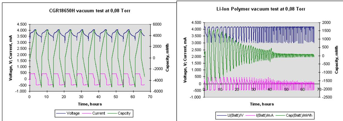
The result of this test is that the Li-Ion Polymer packaging, as expected, wasn't sufficient for low pressure operation. This is due to the fact that the air molecules that are contained in the sandwich construction of the cell are allowed to expand, removing the layers of the cell from each other. This causes in effect the loss in capacity.
