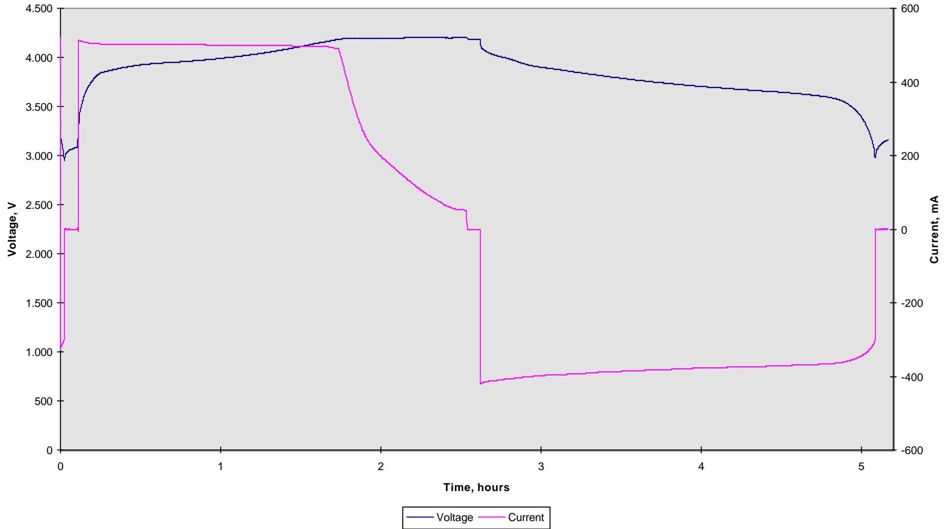
Li-Ion Polymer charge / discharge cycle w/MAX1879 charger
