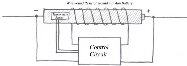
A possible solution is shown in the figure above. The control circuit could be a low power comparator (the heat it dissipates will help heat the battery) that could turn on the wirewound resistor when needed.
