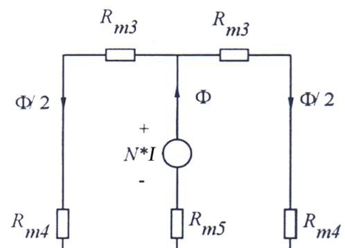
Here the  $R_{m3}$  is the reluctance in the two outer legs,  $R_{m4}$  is the reluctance in the two air gabs for the outer legs and  $R_{m5}$  is the reluctance in the air gab for the center leg.
