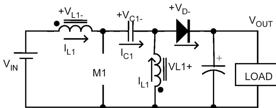
The magnetic energy stored in inductor  $L_1$  is used to charge capacitor  $C_1$ , and the energy stored in  $L_2$  is charging the output capacitor  $C_2$ . The forward diode voltage drop is neglected. The diode could be replaced by a MOSFET to increase efficiency, but it is very urgent that the two MOSFETs never are on at the same time if it happens the output of the converter will be grounded.
