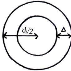
The skin depth  $\Delta$ , is the distance from the surface of the conductor where current can flow.
