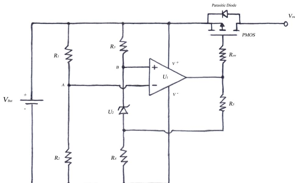
As long as the battery voltage  $V_{bat}$  is above the end of discharge voltage  $V_{end}$  the PMOS will be turned on, when  $V_{bat}$  falls below  $V_{end}$  the PMOS will turn off.
