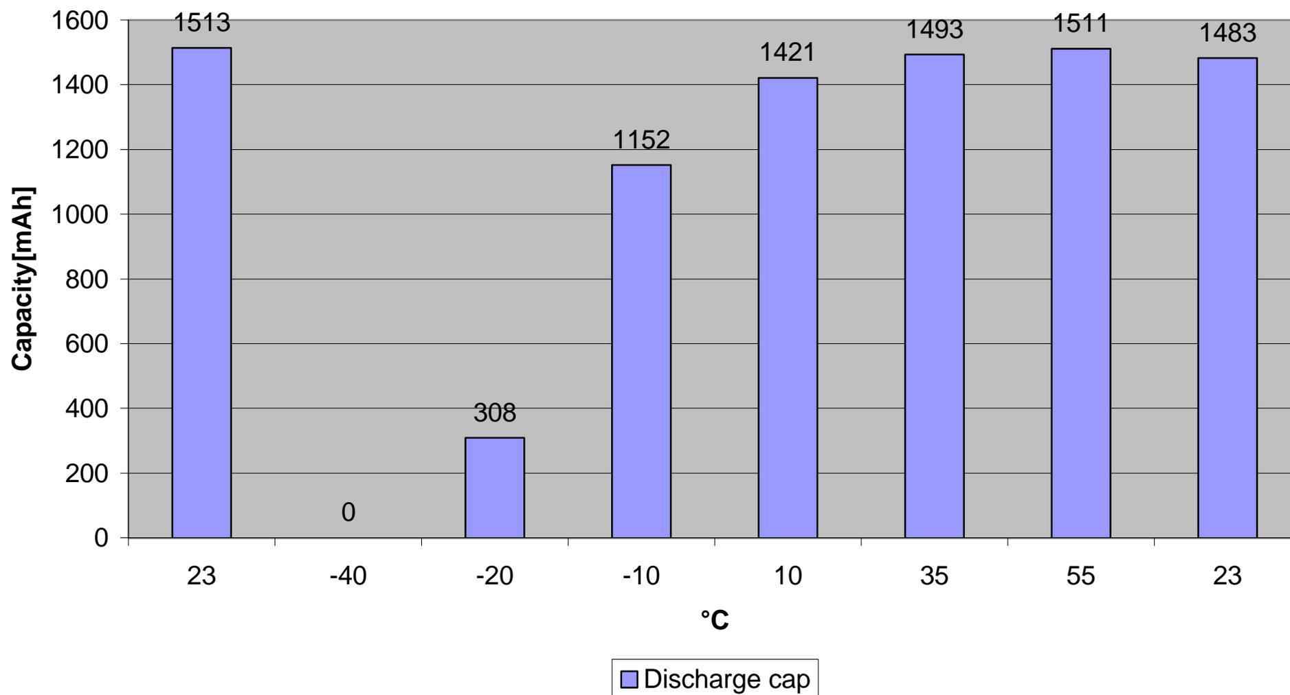
CGR18650H temperature test, discharge
