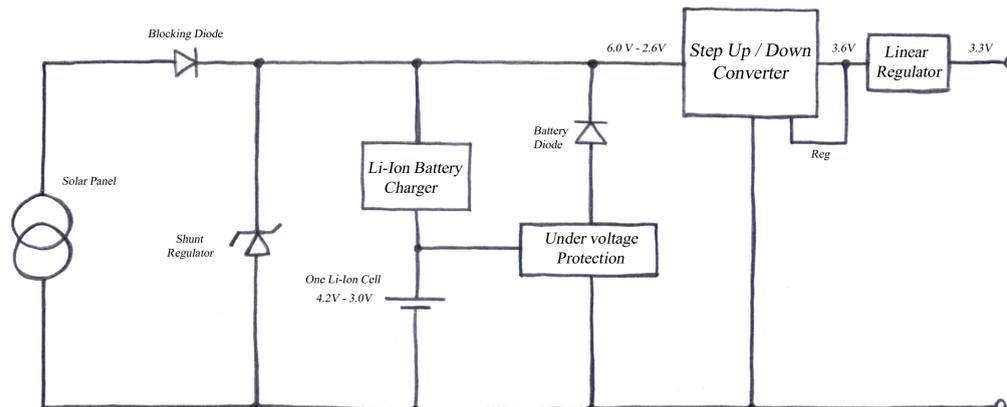
The blocking diodes prevent the solar panels from discharging through each other and the shunt regulator prevents the solar panel voltage from exceeding a value that can destroy the devices attached to the unregulated bus.
