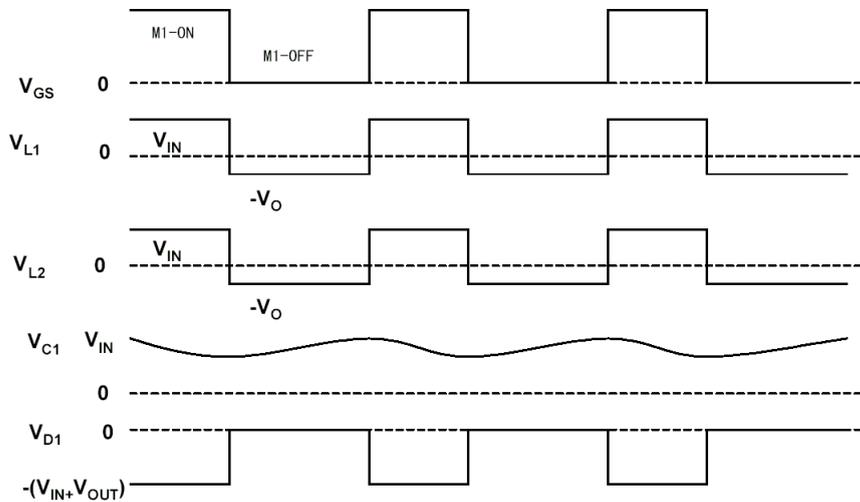
In the on period the voltage across the inductors are equal to  $V_{IN}$  and in the off period the inductor voltages are equal to minus the output voltage because we neglect the diode forward voltage drop.
