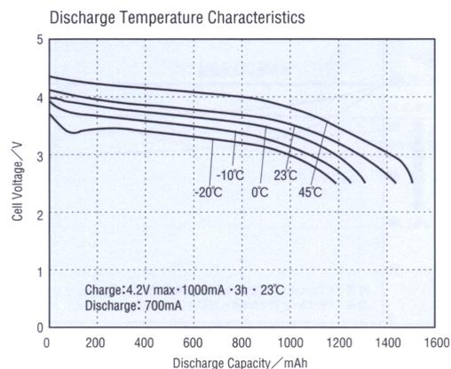
It can be seen that for the -20 °C curve the voltage decreases rapidly in the beginning and then increases again. The decrease is caused by the high internal battery impedance and when current is drawn from the battery the internal chemical activity causes a temperature rise which decreases the impedance and makes the voltage rise again. This phenomena would be even clearer if the temperature curve for -30 °C was shown.
