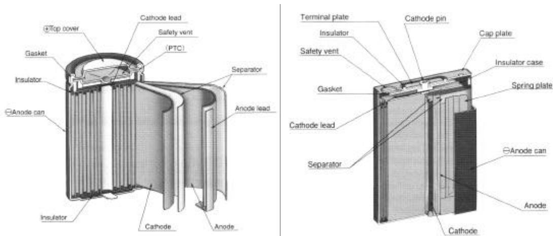
Both containers are made of metal and provide a constant pressure inside the battery even when they are brought into vacuum. So by choosing one of these there will be no vacuum problems.
