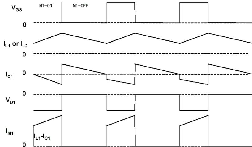
The voltage  $V_{GS}$  just shows the on and off periods of M1 and the diode voltage  $V_{D1}$  show when the diode is reversed and forward biased. The current in the two inductors  $I_{L1}$  and  $I_{L2}$  increases linearly in the on period and decreases linearly in the off period.
