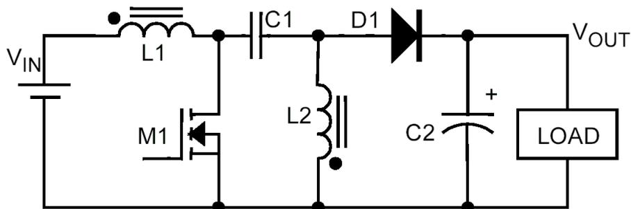
To increase efficiency the two inductors are wound on the same core. When the two inductors are wound on the same core they will not act as two discrete inductors, but as a transformer because of the mutual inductance. Because we use the same inductance value for the two inductors and that the voltage in steady state across the two inductors is the same (explained later) we can assume that the coupled inductors will behave like two discrete inductors like the ones shown in the above figure.
