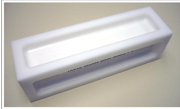
Figure 7.1: CubeSat triple mass model used for P-POD qualification.
