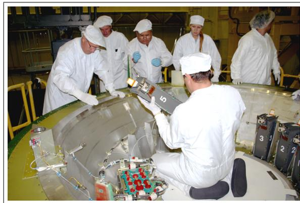
Figure 7.6: Installation of P-PODs onto the SHM.
