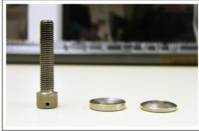
Figure 6.5: Picture of release bolt and spherical washer set.
