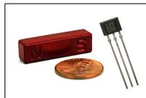
Figure 4.35: A hall effect sensor could be triggered by a magnet in the pusher plate.
