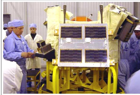
Figure 1.6: Rokot upper stage with CubeSats integrated.
