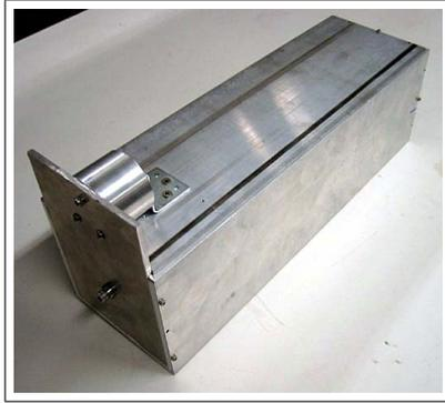
Figure 7.2: Mass simulator for the P-POD Mk. II.
