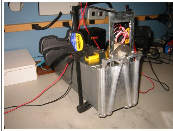
Figure 4.14: Prototype fixture for mounting the Qwknut to the P-POD.
