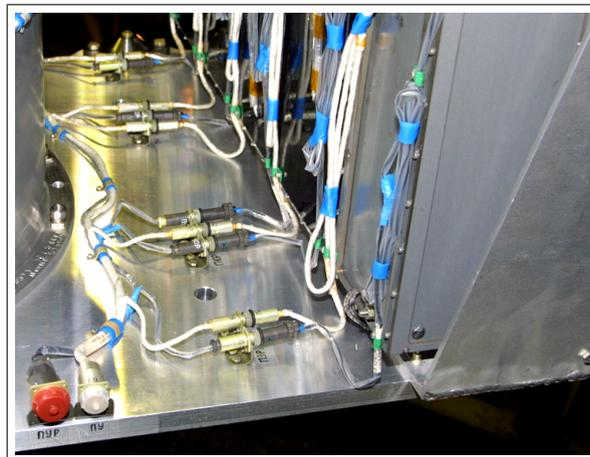
Figure 4.8: Picture of P-POD electrical connections.
