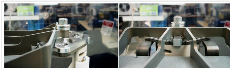
Figure 6.2: Two side views of the Qwknut and release bolt.
