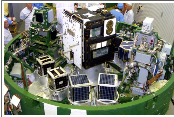
Figure 1.9: Integrated Dnepr space head module for fourth launch.
