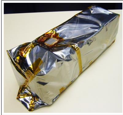
Figure 7.4: P-POD bagged for cleanliness, ready for testing.
