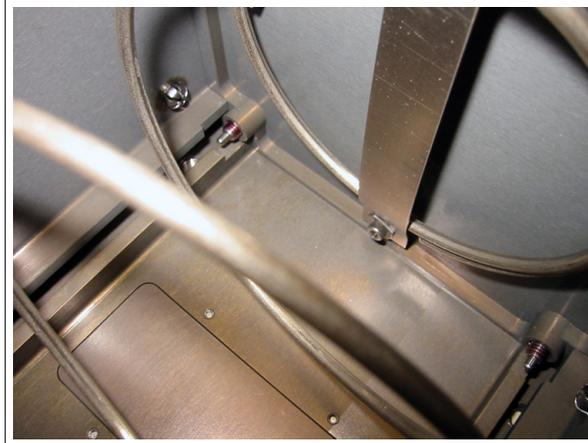
Figure 4.31: Internal P-POD rails cut to accommodate kick springs.
