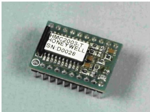
Figura 3.15: *Il magnetometro Honeywell HMC2003*
