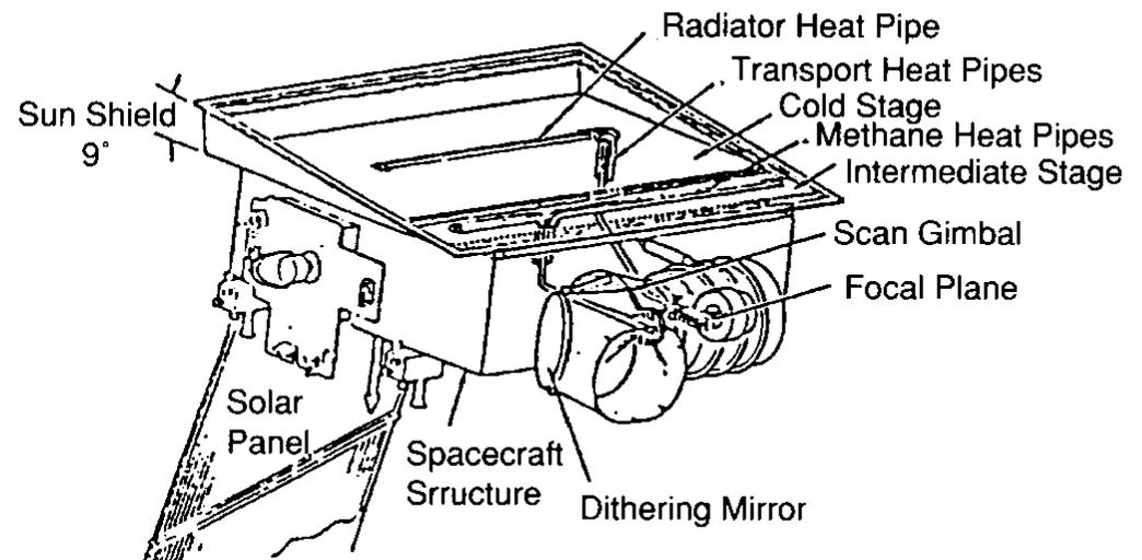
The cold stage rejects 5 W heat at 70 K from a  $\approx 1 \text{ m}^2$  surface
