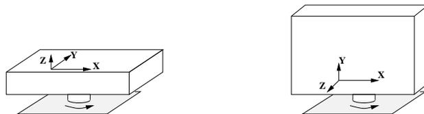
Figure L.1: To the left the magnetometer is rotated in the X-Y plane In the right figure the magnetometer is rotated in the X-Z plane
